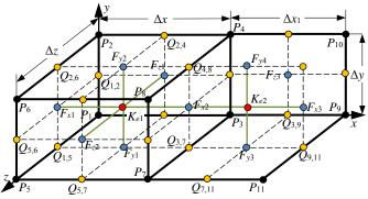
Fig. 1. Characteristic points for a hexahedral element.
